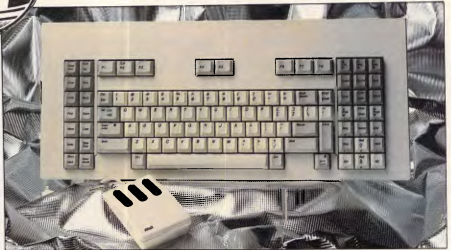
The 103-key keyboard features hard and soft defined function keys
